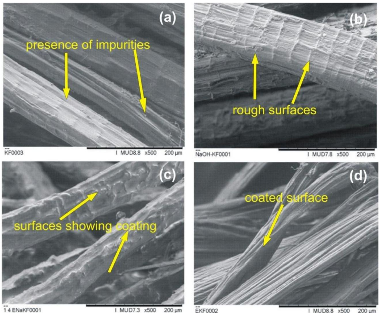
**Figure 3:** Morphology of (a) raw kenaf fibre (KF), (b) NaOH treated kenaf fibre (NKF), (c) epoxy coated-NaOH treated kenaf fibre (ENKF) and (d) epoxy coated kenaf fibre (EKF).
