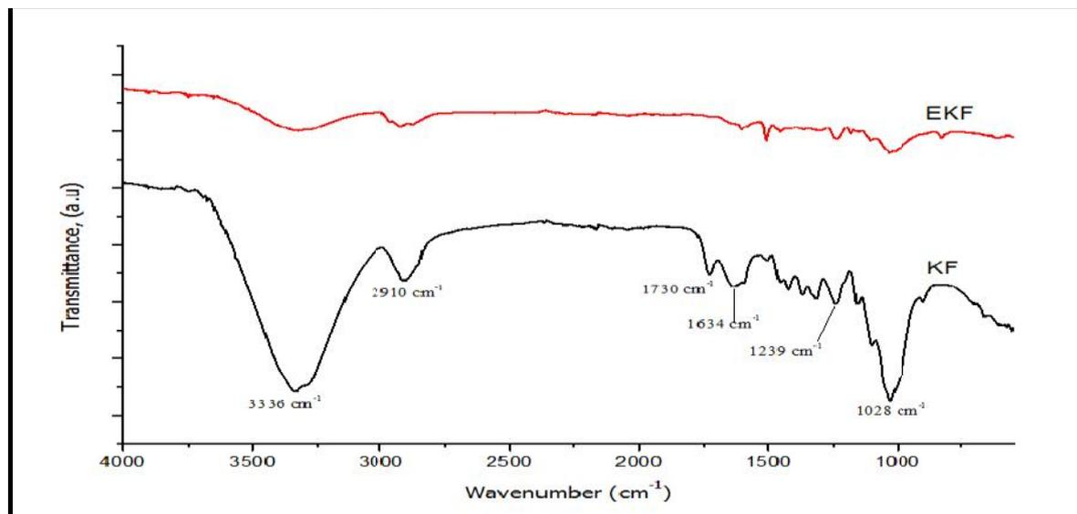
**Figure 2b:** The Combined spectra of raw kenaf (KF) and epoxy coated kenaf (EKF).
