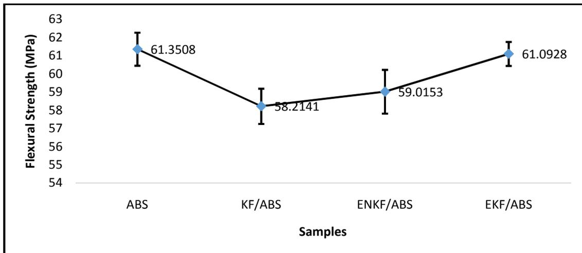
Figure 5: Chemical treatments effects on the flexural strength of kenaf fibre filled ABS composites at 10 wt% constant fibre loading.
