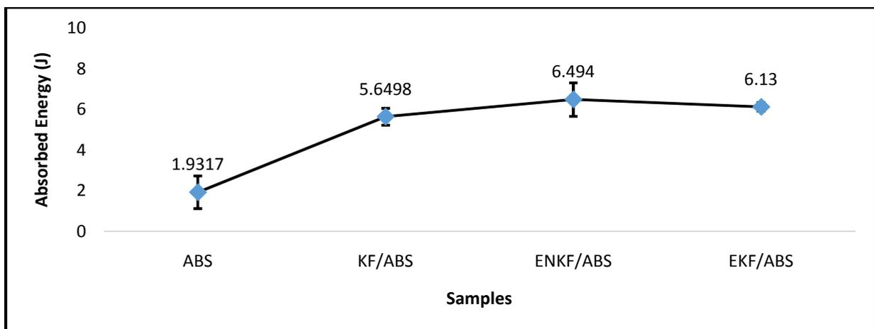
**Figure 8:** Chemical treatment effects on the impact absorbed energy of kenaf fibre filled ABS composites at 10 wt% constant fibre loading.
