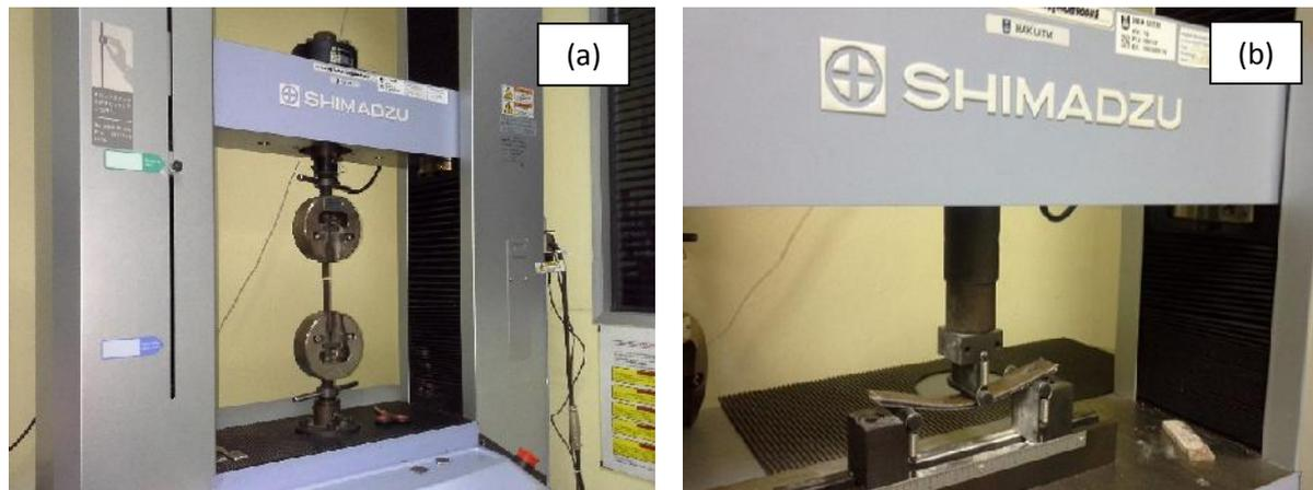
Figure 1: (a) Tensile testing procedure showing the test specimen clamped in the SHIMADZU Universal Tester and (b) Flexural testing procedure showing the 3-point bending configuration.
