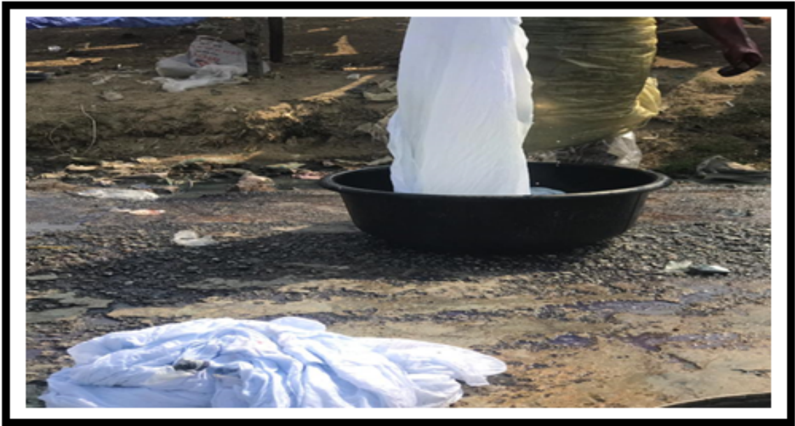
Figure 1: Continuous movement of fabric relative to dye liquor (Remove pic) (the Figure is very important to depict how the dyeing is carried out)
