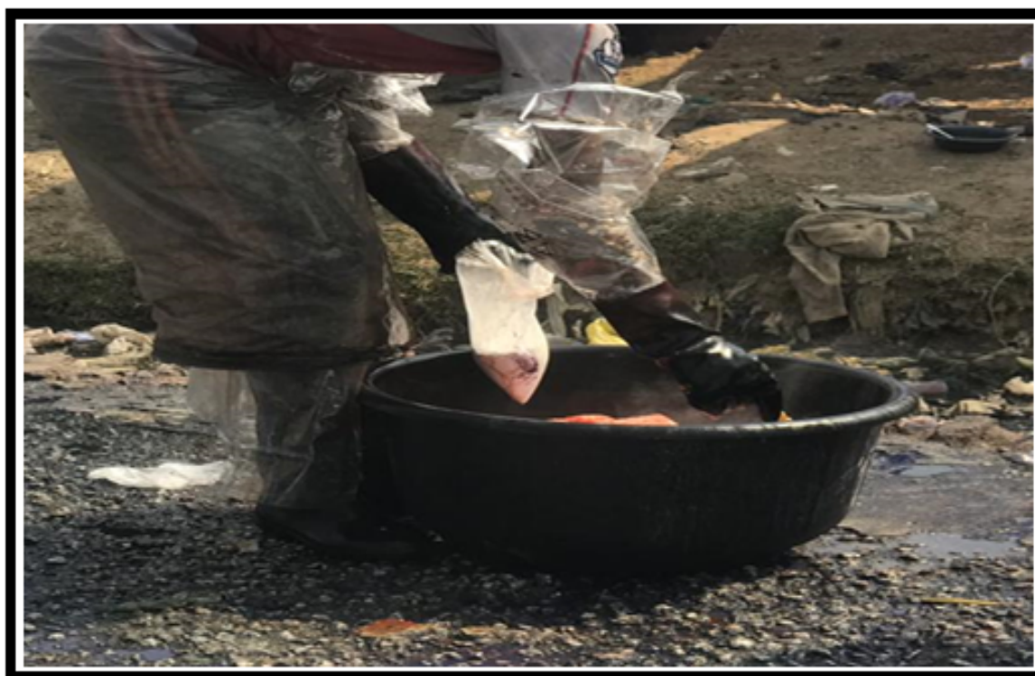
Figure 4: Metered addition of dye and hydros in the course of dyeing (Remove picture) (those pictures are very important in a survey to show the actual processes)
